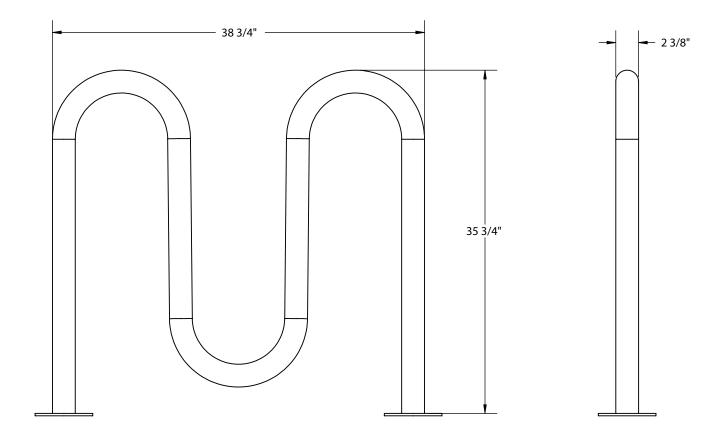
Recommended Surface Mount Hardware: 3/8" x 3-1/2" Concrete Expansion Anchor Bolts
